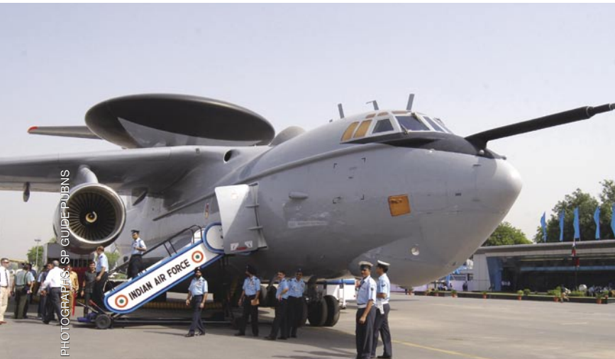
E-SPY: The IAF's AWACS is equipped with Phalcon radar on an IL-76 platform
